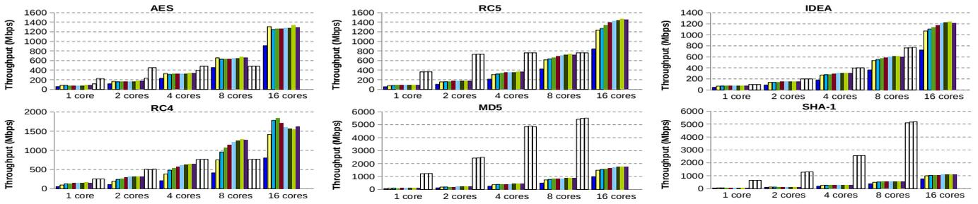
Fig. 9. Combined throughput for 1-8,16 streams per core on 1-16 cores (1-256 streams total). IXP2800 performance in leftmost 3 bars at each core group.
