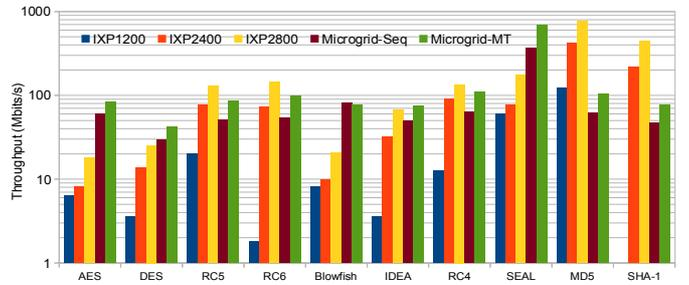
Fig. 8. Throughput for one stream on one core.
