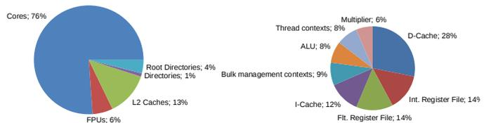
Fig. 3. Chip area breakdown: entire grid (left), per core (right).
