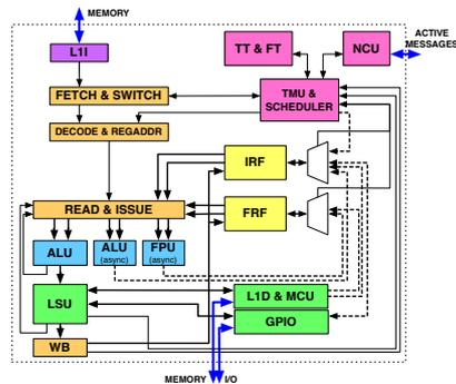
Fig. 1. Core micro-architecture.
