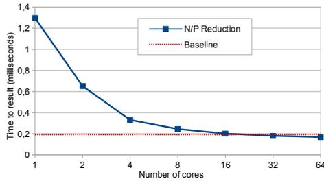
Fig. 5. Scalability of a N/P reduction of 64k floating-point values.
