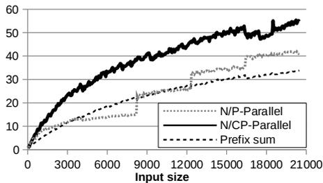
Fig. 6. Speedup of various parallel reduction strategies on 64 cores.
