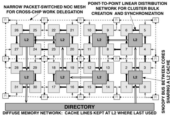
Fig. 2. Microgrid of 32 cores.
