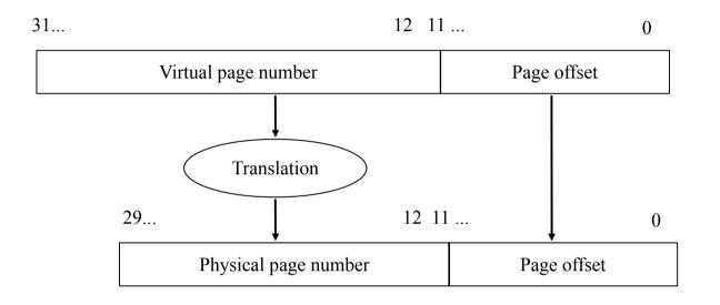
This shows address mapping from a 4 GiB virtual address space onto in a 1 GiB physical address space using 4KiB memory pages
