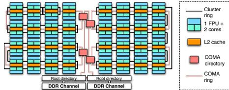
**Fig. 1.** Functional diagram of a 128 core Microgrid.
