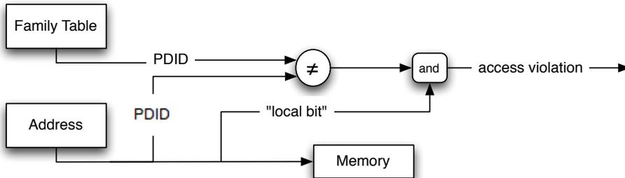
Figure 2: Implicit TLS protection mechanism
