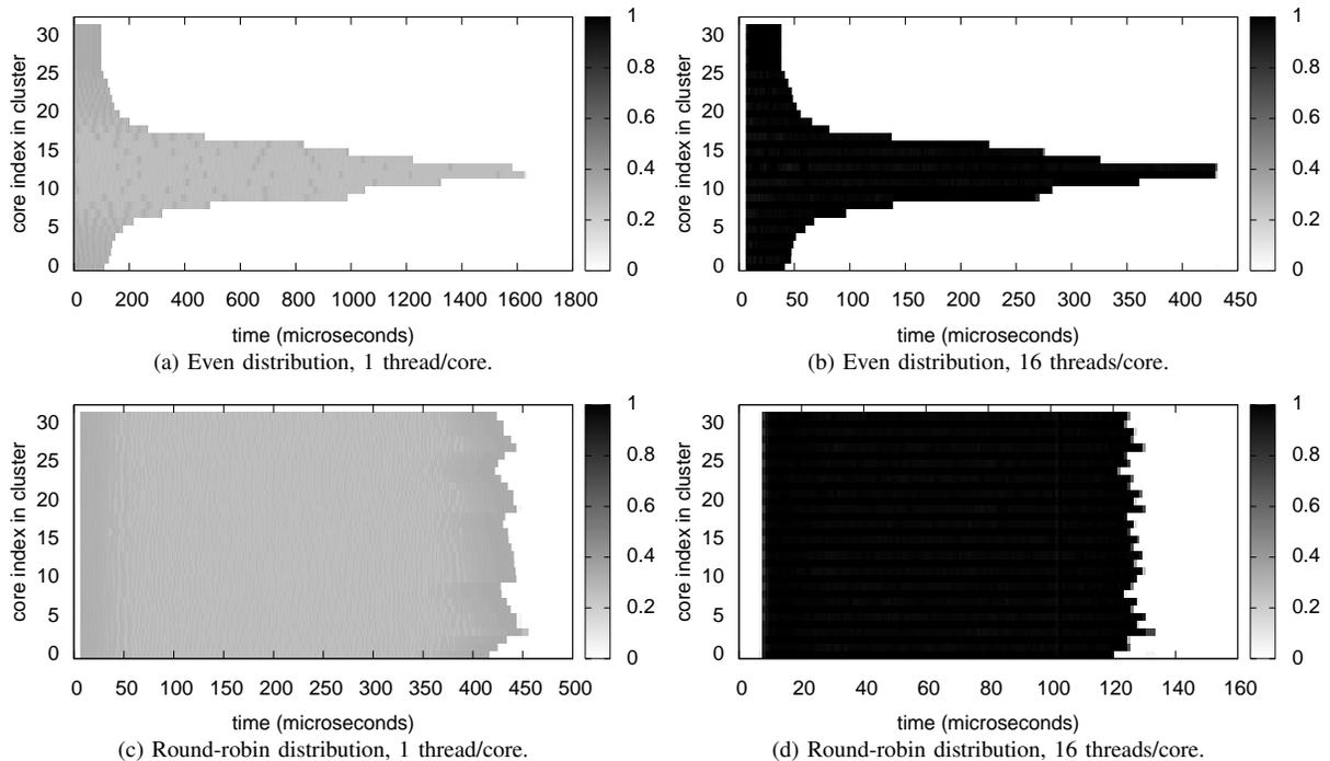
Figure 3. Per-core IPC over time for the Mandelbrot set approximation, running on 32 cores.
