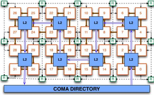
Figure 6. Example MGSim configuration: a 32-core Microgrid.
