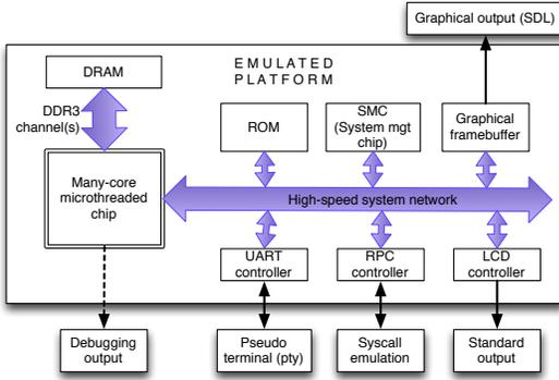
Figure 7. Example MGSim configuration: a full-system Microgrid platform.
