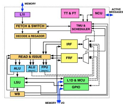
Figure 2. D-RISC core micro-architecture, as simulated in MGSim.
