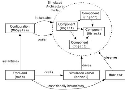
Figure 5. Entity-relationship diagram of an MGSim simulator.
