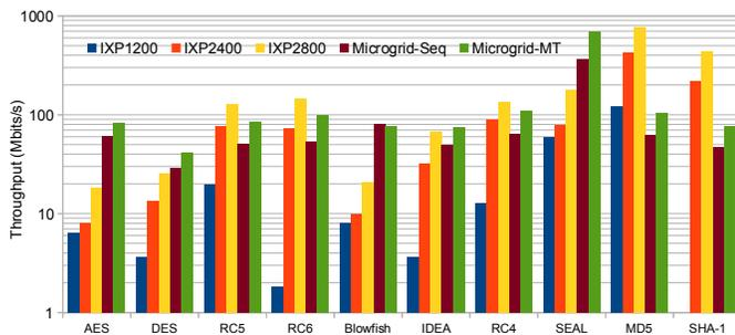
Figure 4. Throughput for one cryptographic stream on one core.
